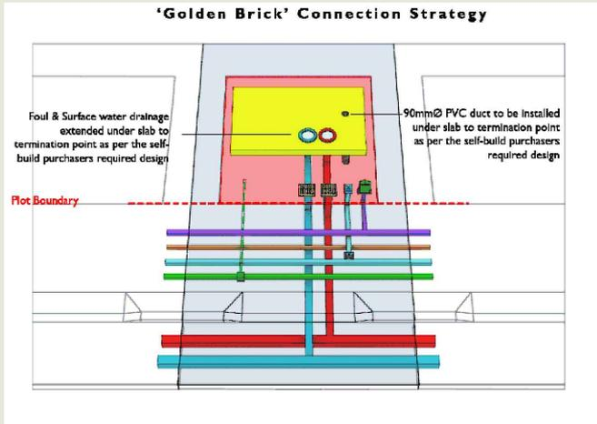
Self-build purchaser to supply and install a standard 25mm conduit through the cavity wall at the point that is vertically above the end of the service duct. External capping 25A and connector Bend 4 should be fitted as required.
