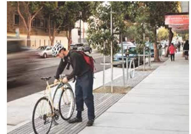
ABOVE Neutral, restrained & accessible hardscape on Gough Street in San Francisco. All street clutter (e.g. cycle stands, lighting columns, benches, bins etc.) is confined to a 'functional strip' that separates vehicular from pedestrian zones in order to maintain clear & legible routes for passing traffic. Intermittent street trees also sit within this strip, adding a welcome dose of greenery to the otherwise hard, urban treatment of this space. Gough Street, San Francisco; TAKEN FROM http://goo.gl/HwFBC8
